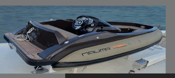
The Tenderlux 390/380 is the smallest model of the Naumatec RIB range. Molded with vinylester resins, using the infusion technique, it features a low dry weight yet a wide and particularly comfortable onboard space for a tender of its size. As for the entire Naumatec range, the product quality is kept high through the use of first choice teak, special paints and upholstery made with modern tech, exotic fabrics and elegant colours.
